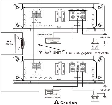
When utilizing the dual amplifier configuration it is important to note that the connected speaker load can be no lower than 2 ohms. Connecting a lower impedance load can damage the amplifier and void your warranty
